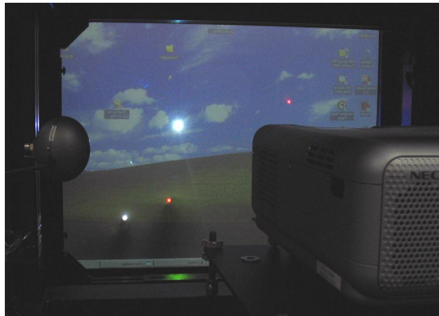
Figure 7 View from inside a MAD Box. Central bright spot is reflection of projector bulb. Top right red dot is laser pointer spot. Bottom left spots are white and red LED lights.
